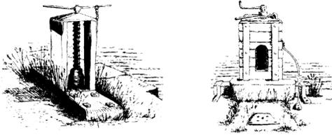
Two drawings of typical Leeds & Liverpool Canal ground paddles, called 'box cloughs'. Every canal had its own particular style.
