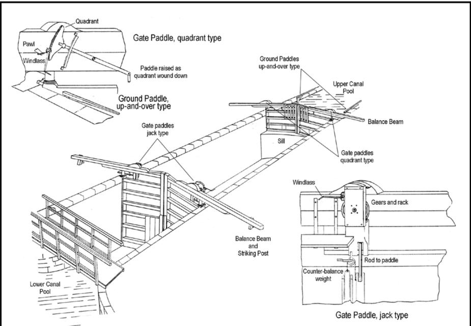
A drawing of a Leeds & Liverpool Canal lock showing further types of paddle gear. On the up-and-over type, the horizontal bar is raised at one end, turning it through 90 degrees, and this turns the vertical lever to which it is attached, opening the paddle hole.
