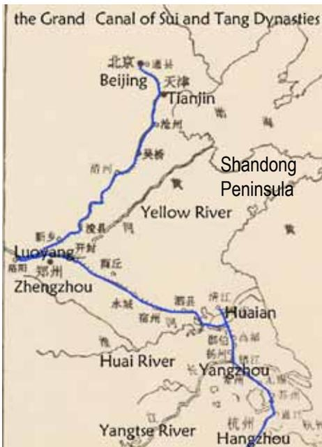
Left: The earliest route of the Grand Canal in China, pre-1324 AD, with the Yellow River running to the north of the Shandong Peninsula. The river carries vast amounts of silt, but the canal was kept relatively silt free as it was fed by the clean waters of the Huai River, and this affected the design of the locks built on this section of canal.
